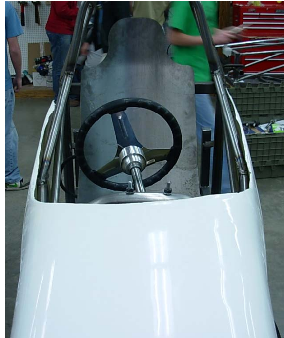
This is a picture of the steering wheel and the seat (not yet welded on) and the top of the fiberglass body.
