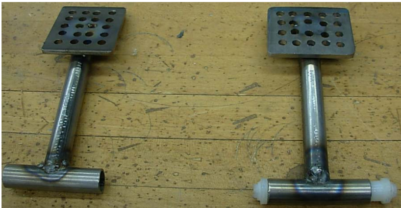
The pedals we have created and assembled. Both pedals will eventually have bushings (the white plastic inserts) which will make mounting the pedals easier.
